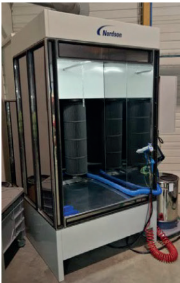
Cabine application poudre Dimension : H1250 mm x L1000 mm x P500 mm
